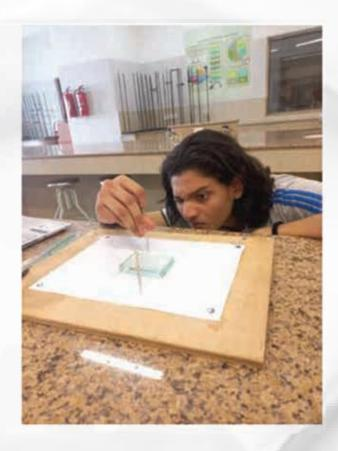
MYP V Physics students conducted an engaging experiment to determine the refractive index of glass, deepening their understanding of light behavior. The refractive index, a fundamental property of materials, measures how much light slows down or changes direction when passing through a medium compared to a vacuum.
